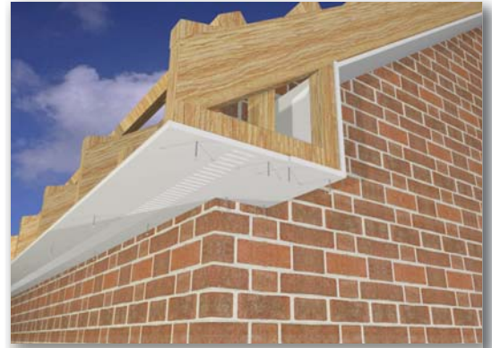
Fig 20a. Typical GPBV soffit installation.
