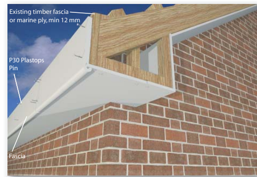
Fig. 17. Standard over-fascia installation.
